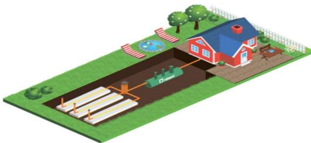
Figure 6. Installation scheme of a septic tank
