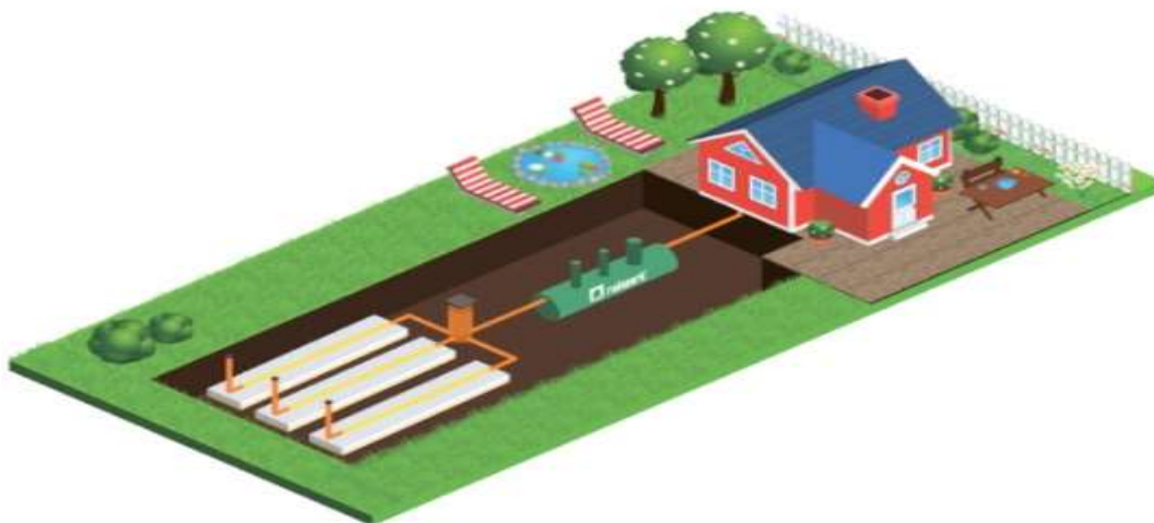
Figure 6. Installation scheme of a septic tank
