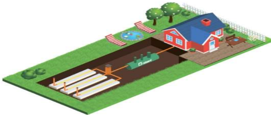
Figure 6. Installation scheme of a septic tank
