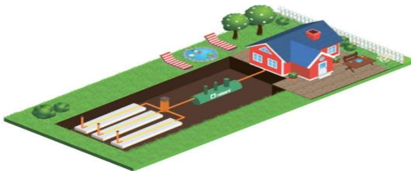
Figure 6. Installation scheme of a septic tank
